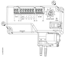
IP54 box mounting: The IP54 rated APS can only be mounted as shown.
